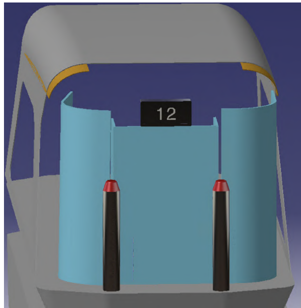
Figure 3.20: CAD model of the counting system with lights and countdown for the indication when maximum amount of passengers has been reached.
