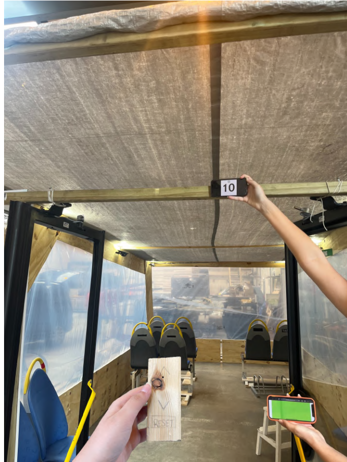
Figure 4.5: Setup of the counting indicators: countdown screen and lights to alert passengers when maximum capacity is reached.
