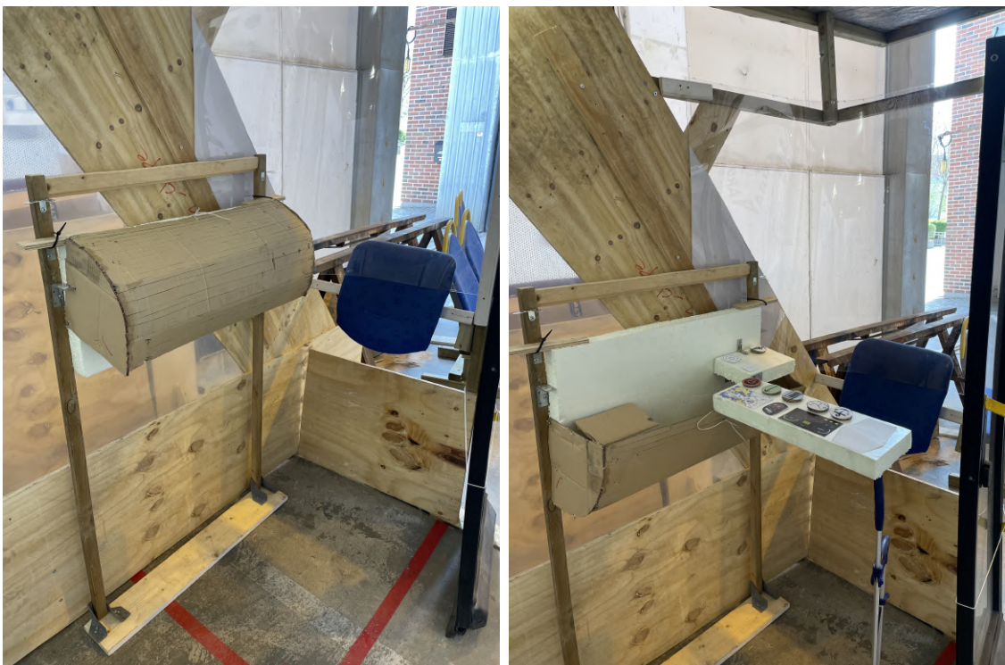
(a) Buffet cover pulled closed over the wall-mounted, space-saving solution. (b) Dashboard folded out for usage of the space-saving solution.
