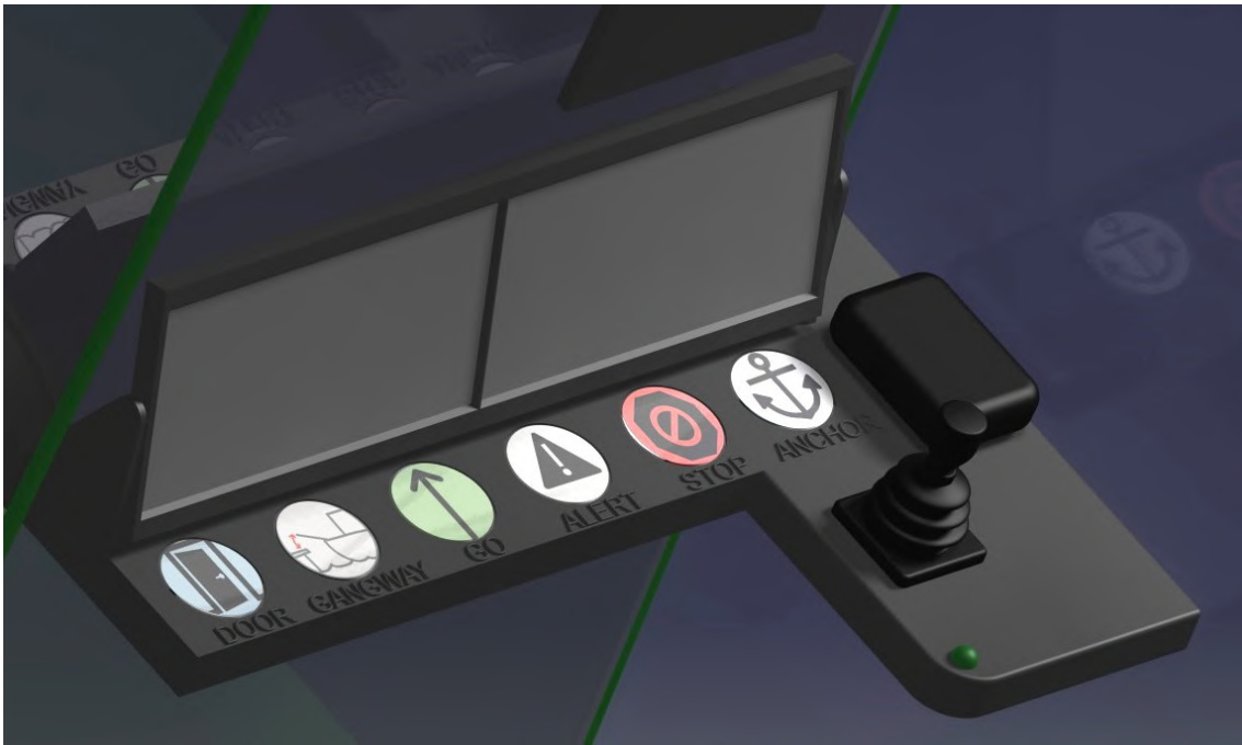
Figure 5.3: A close-up shot of the dashboard, showcasing the compact design, tiltable screens, button decals and embossing, and integrated joystick.
